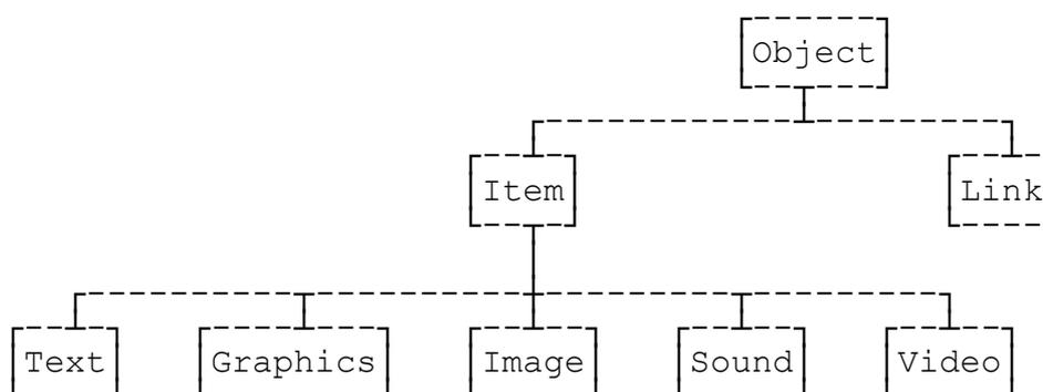
Nodes in this tree structure correspond to classes. Children nodes represent subclasses and parent nodes represent superclasses. Each class inherits all the data variables and the methods defined for all its superclasses up to class Object and has some data variables and methods of its own. Data variables and methods are either inherited without change or inherited and redefined.
